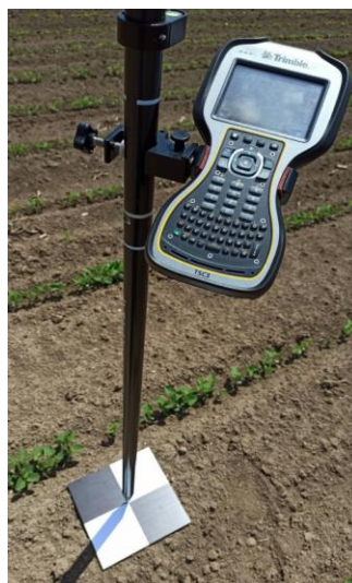
Slika 3. Merenje kontrolnih tačaka Figure 3. Measuring of control points
